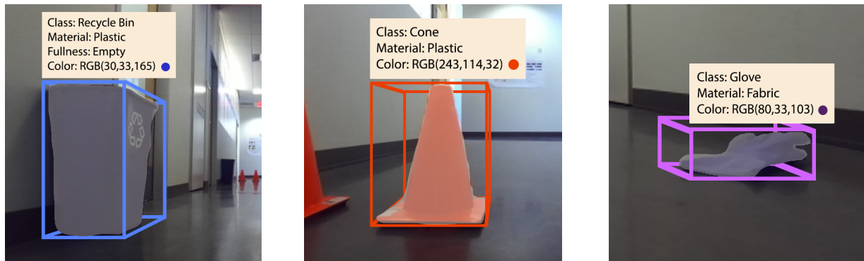
Figure 1. Object detection and characterization for three worksite objects, using the proposed object characterization framework and algorithm.
