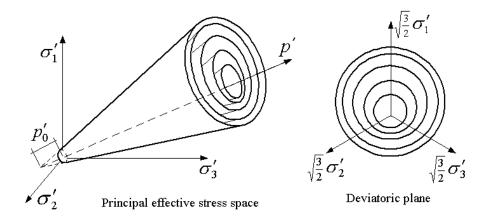
Figure 1 - Conical yield surface in principal stress space and deviatoric plane
