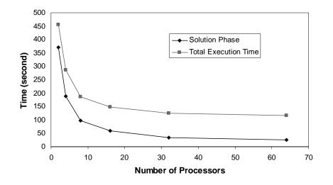
Figure 4 – Solution times for the soil-pile interaction model
