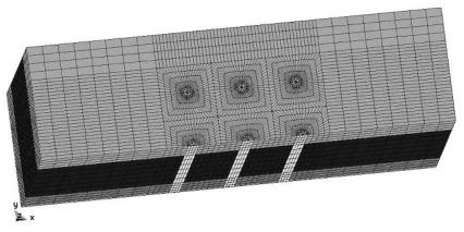
Figure 3 – A soil-pile interaction finite element model
