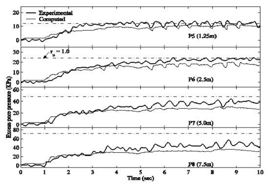
Figure 7: Recorded and Computed Excess Pore Pressure Time Histories
