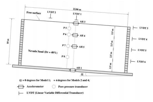
Figure 5. General Configurations of Test Model in Laminar Container
