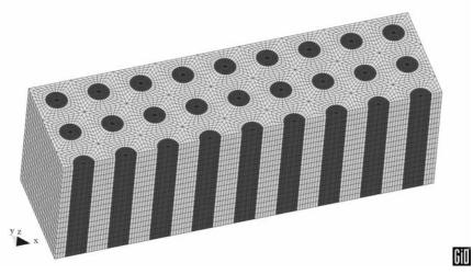
Figure 4. Finite Element Model of the Stone Column Centrifuge Test
