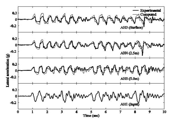
Figure 6: Recorded and Computed Lateral Acceleration Time Histories
