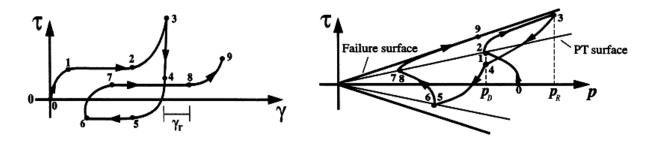
Figure 2. Constitutive Model and Effective Stress Path under Undrained Shear Loading
