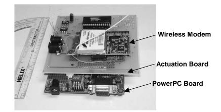
Fig. 2. Three printed circuit board stack assembled as a single wireless active sensing unit prototype
