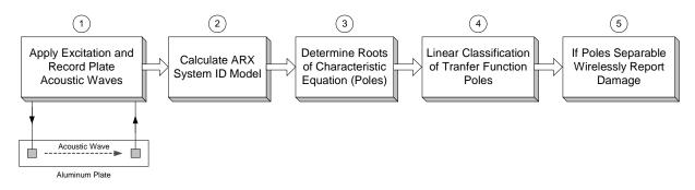
Fig. 6. Embedded damage detection methodology based on the migration of transfer function pole locations
