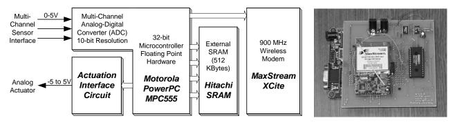
Fig. 1 Architectural design of the wireless active sensing unit
