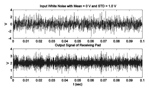
Fig. 5. (Top) white noise excitation with a 1.0 V standard deviation; (bottom) measured response of the aluminum plate
