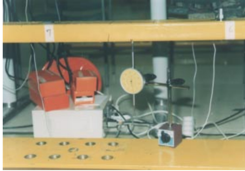
Figure 6.8: Actual damage introduced to the grid-type bridge structure
