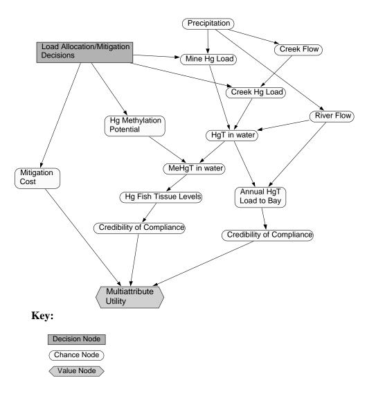
Figure 5 - Influence Diagram for Mercury Load Allocation/Mitigation Decisions for a Small Watershed Impacted by a Mercury Mine Site and Mine Wastes.
